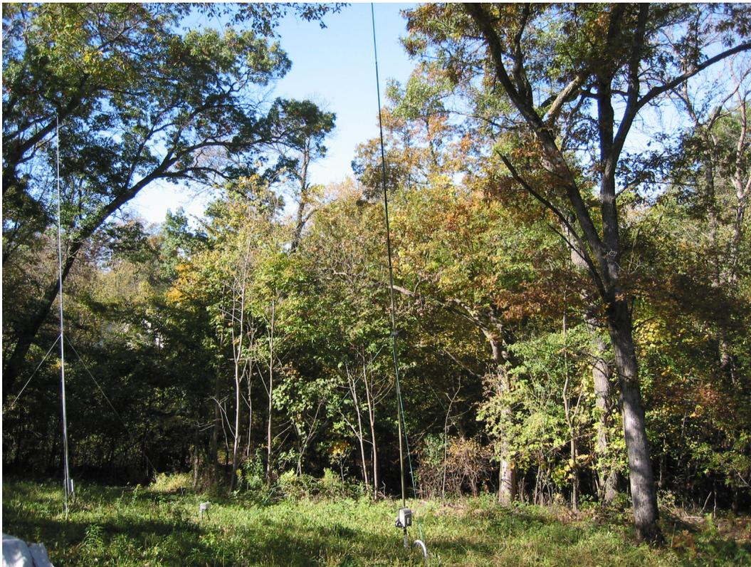
**#1: Phased verticals aimed 30 degrees for EU, broadside to Asia. The DXE 40m is left while the 80-6m BigIR MK3 is on the right. Note the phase switch in-between the two**
