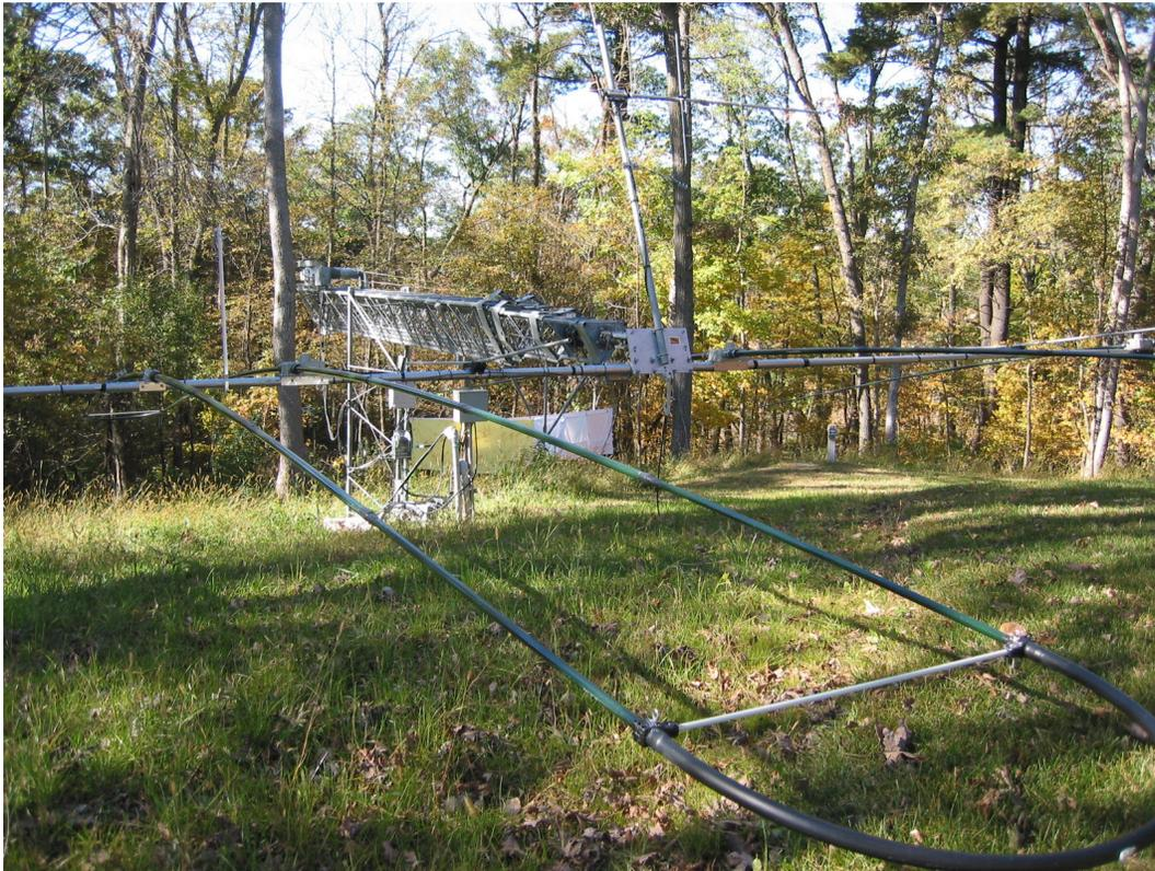
**#2:** SteppIR on the LM470 tilt over tower. Shown in foreground is the 40/30 loop without the truss assembly.
