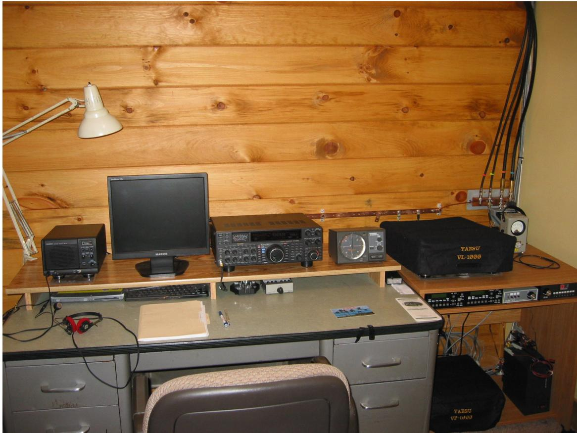
**#7:** The station in the basement shows the FT-2000 and G2800 rotor control. To the right of that is the VL-1000 PA deck. Note the VP-1000 PS for it is below it on the 'computer' stand. I found that the SteppIR controllers fit perfectly into the 'keyboard' nook! Next to the vertical controller is the Comtek phase switch. To the far right is the DXE antenna selector. Note the common bus bar for the coaxes and transceiver/amp.
