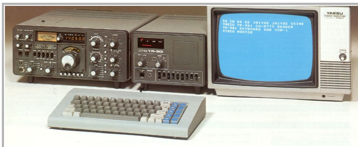
RTTY 33 years ago - Circa 1979 - YAESU YR-902DM Transceiver, and YAESU YR-901DM RTTY Reader.
