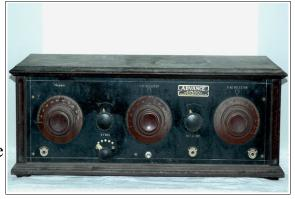
vauum out. The receiver uses five tubes, an AX201A, two CT201A, one CX301A, and an un-identifiable mystery tube, although it has one thing that none of the others have and that is S R & Co., 10 25, stamped on the metal base. I suspect these receivers were sold by Sears, Roebuck & Co. and this particular tube was manufactured in October of 1925. Advance Electric equipment was manufactured in Milwaukee, Wisconsin. Larry - KØIS
