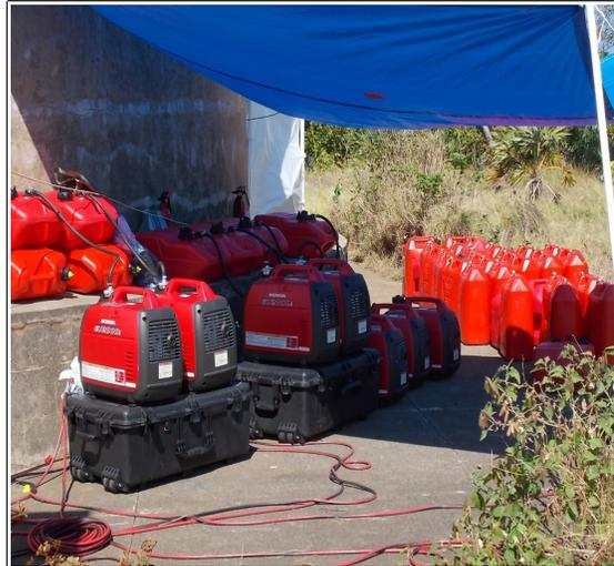
**Honda 2000 watt generators, one for each station (7). Under full load, they used just under 1 qt/hour. When using low power in the “eco mode”, even much less fuel was consumed.**
