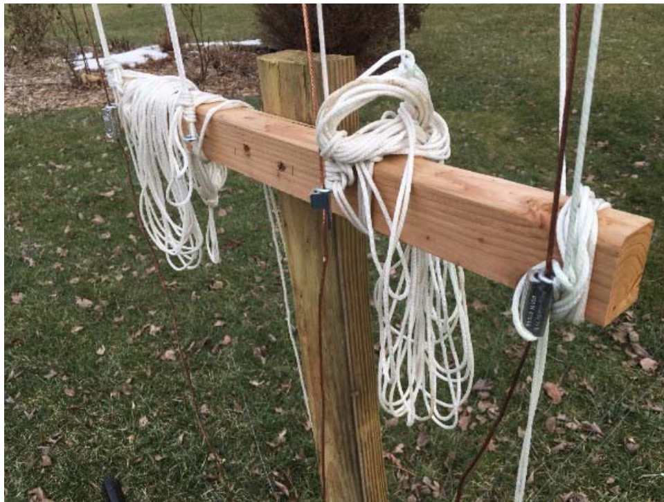
Each element wire has a splice block fastened to it to give me something to pull tension against.
