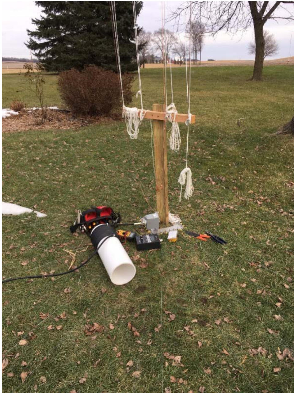
Lower mounting bracket. White ropes run to pulleys on a 4' bar hoisted into the tree.
