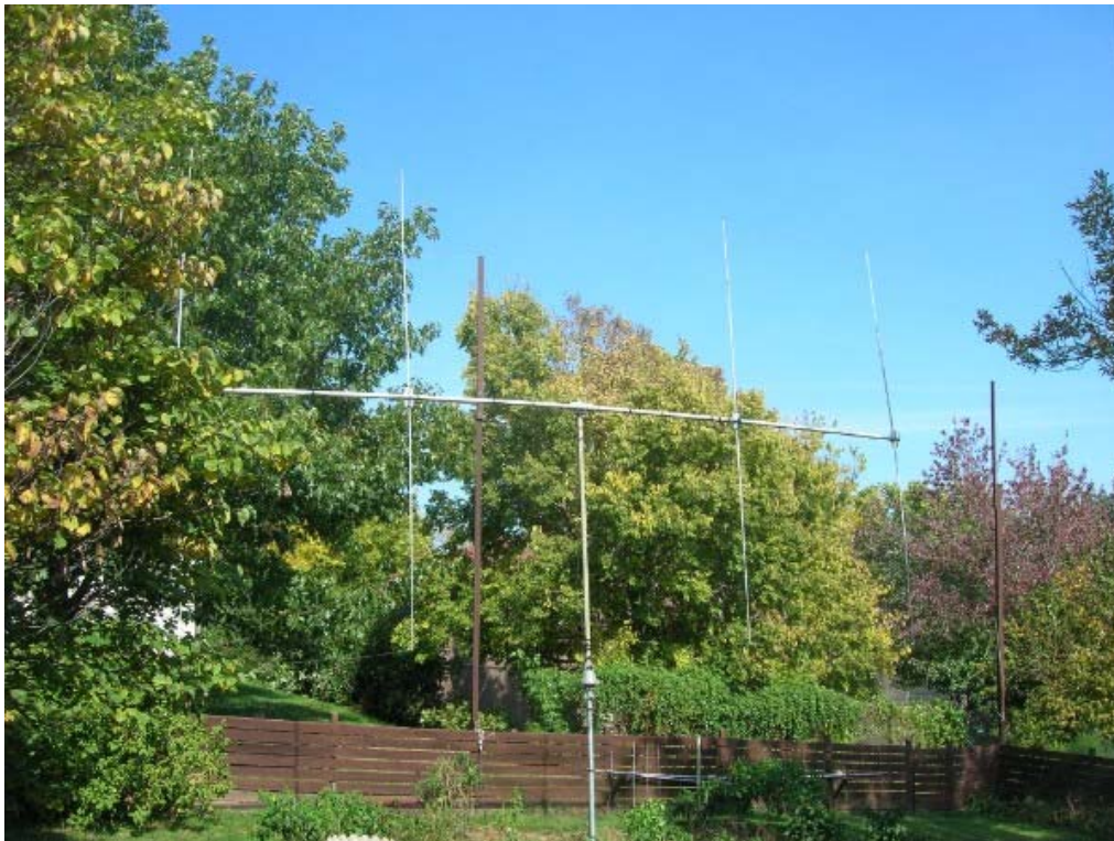
The rotatable Waller flag, together with a rotatable magnetic loop mounted on a 4 ft. mast have been respectable receiver antennas on
