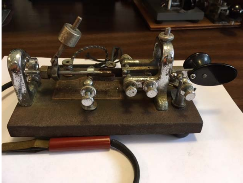
Bob Denniston's 1955 Vibroplex Standard - modified with his Vertical Pendulum.
