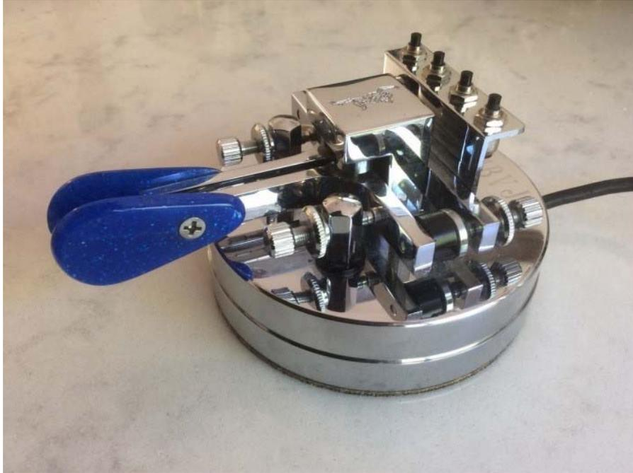
Lance Johnson Engineering later developed the MR-1 bracket with four push buttons for the Mercury Key that interface with the KC-1 allowing selection of four pre-programmed memory options. I bought my KC-1 and MR-1 from Lance Johnson which was owned and run by Steve Gecewicz K0CS. I used this set-up many times in contests and at special event stations. I still have the keyer, manual and application guide.
