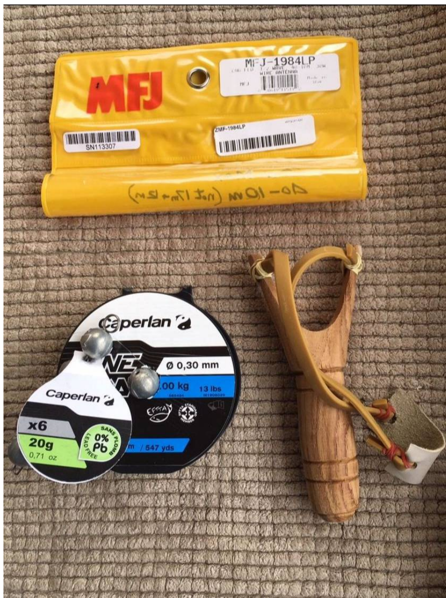
The antenna kit. Slingshot, Fishing Weights, monofilament line and little MFJ end-fed.
