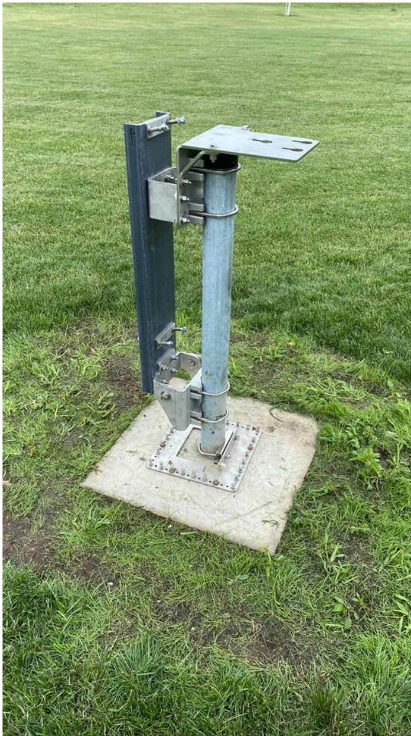
Attached to the mounting pipe. The plate on the top is where the winch will mount. Holes are slotted so you can remove the winch when not in use so the web belt doesn't degrade from UV exposure.
