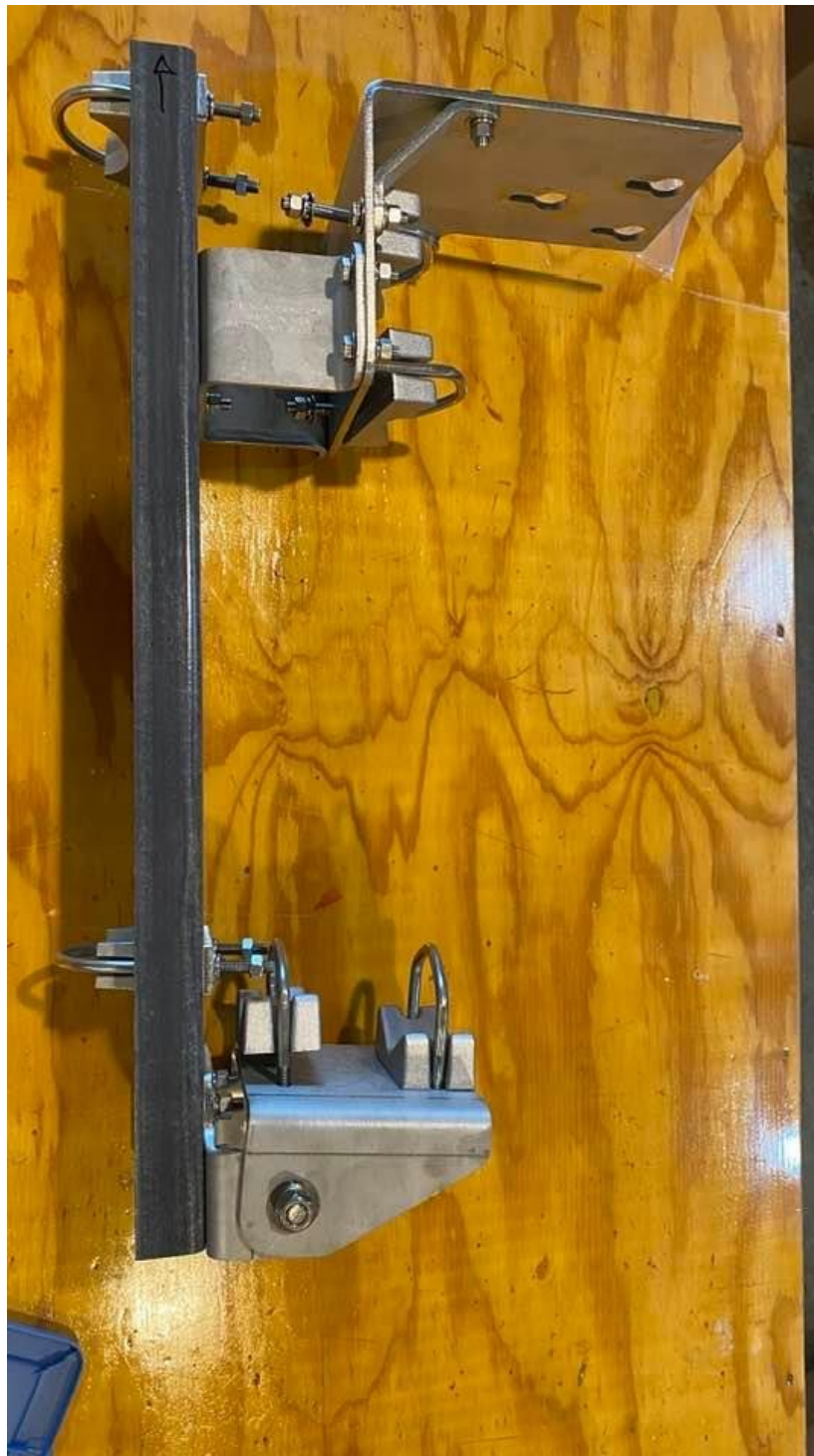
This is the tilt mount ready to attach to the mounting pipe. The channel on the left is non-conductive.
