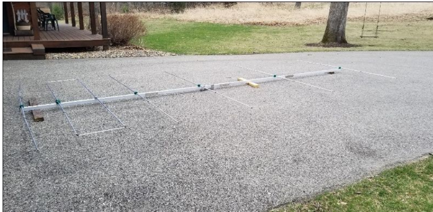
The InnovAntennas LFA MAX 6 Element 6 Meter Yagi on a 19' boom
