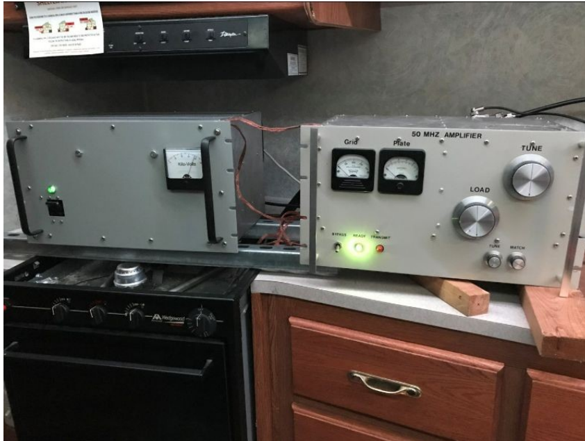
My HB 6-Meter PA and PS – 1400 Watts Output
